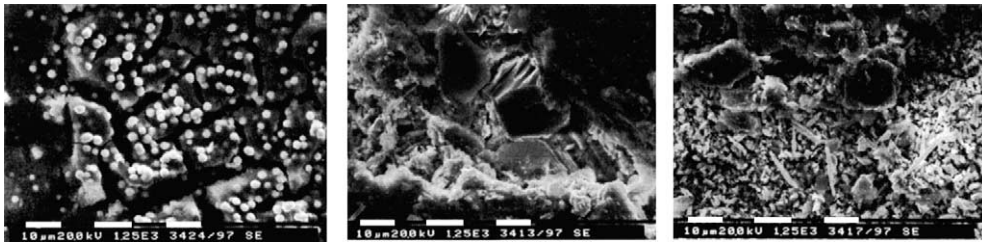
Fig. 3. SEM pictures of the top of the reaction layer of glasses SON68 (left) and WG124 (middle and right) after corrosion in the CERBERUS test. Left we see a Zn, S phase (the white spots), in the middle an \text{SiO}_2 phase (middle of the picture) and in the right picture various phases, with high Ba, Fe and S concentration.
